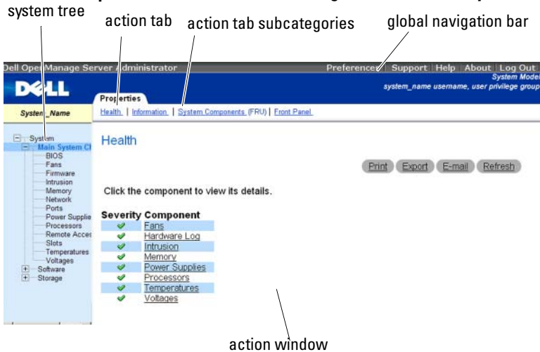
Figure 5-1. Sample Server Administrator Home Page — Non-Modular System
